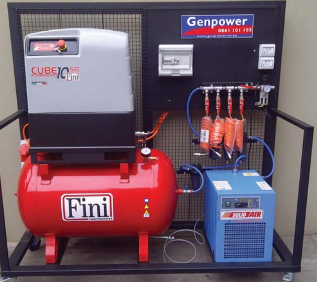
Portable Rotary Screw compressor for spraying of Polyurea at ABSA building.
